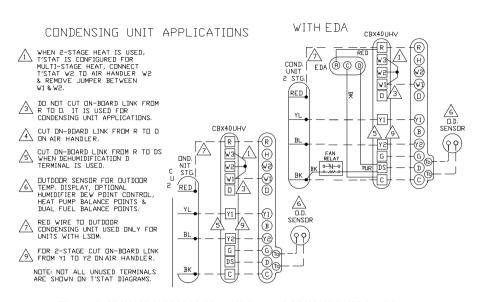
Figure 4. CBX32MV-XXX-230-06 or Higher and CBX40UHV Wiring Diagrams (Condensing Unit Applications)
