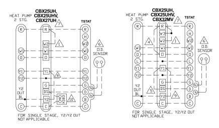
Figure 10. Thermostat Wiring Diagrams (continued)
