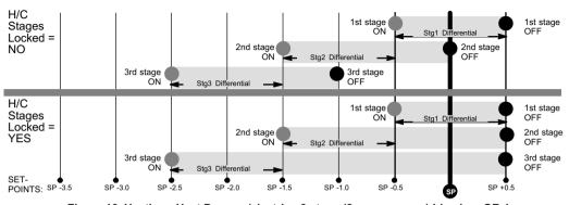
Figure 16. Heating - Heat Pump w/electric - 3 stage (2 compressor / 1 backup OR 1 compressor / 2 backup)
