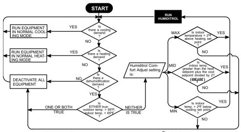
Figure 22. Thermostat Operation with Humiditrol® EDA Enabled
