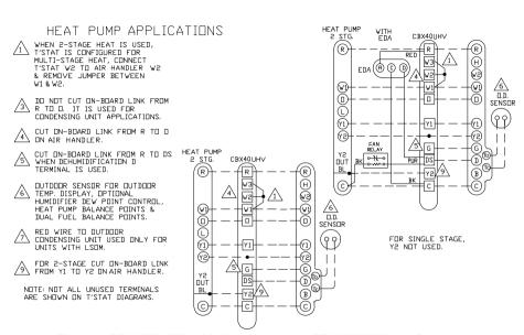
Figure 5. CBX32MV-XXX-230-06 or Higher and CBX40UHV Wiring Diagrams (Heat Pump Unit Applications)
