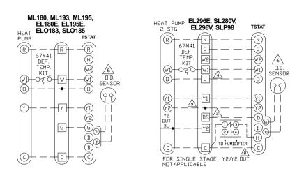
Figure 11. Thermostat Wiring Diagrams (continued)
