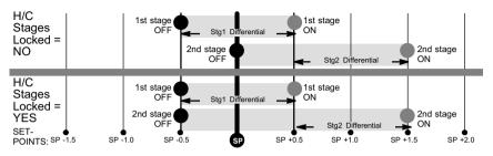
Figure 14. Cooling - 1 or 2 stages
