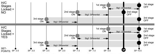
Figure 20. Heating - dual fuel - 3 stage (2 compressor / 1 backup)
