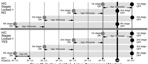
Figure 21. Heating - dual fuel - 4 stage (2 compressor / 2 backup)
