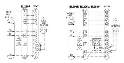
Figure 9. Thermostat Wiring Diagrams (continued)
