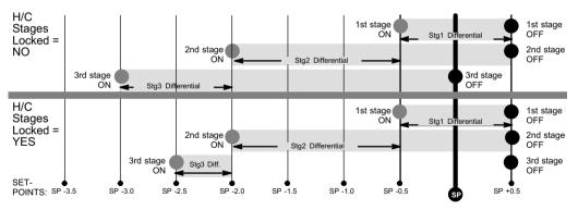
Figure 19. Heating - dual fuel - 3 stage (1 compressor / 2 backup)
