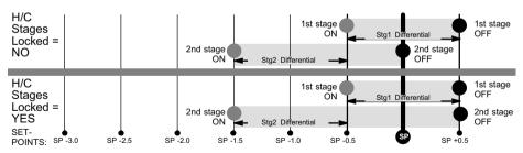
Figure 15. Heating - Non-Heat Pump or Heat Pump w/o backup heat - 1 or 2 stages
